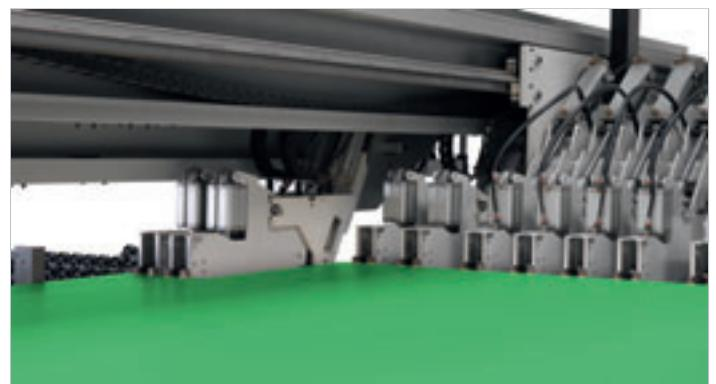
According to the cutting pattern, the two idle slave grippers can be linked, individually or together, to either pusher.
