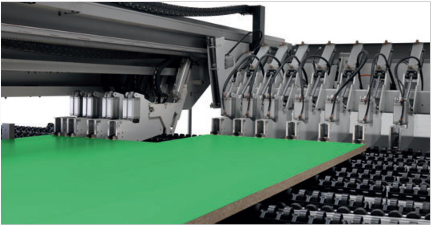
Device for simultaneous execution of staggered cross cuts, made with two completely separate pushers. Each pusher can choose to select two idle slave grippers (not powered) completely independently, based on the strips width to be cut. This unique solution allows to modulate the width of the two pushers and their working area (patent pending).
